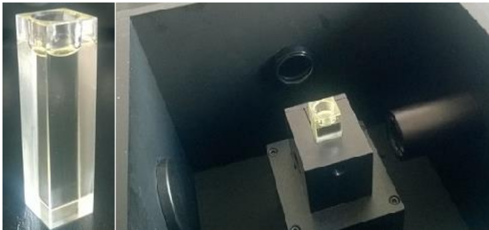
Figure 2. Quartz cuvette and its placement in the measuring device
