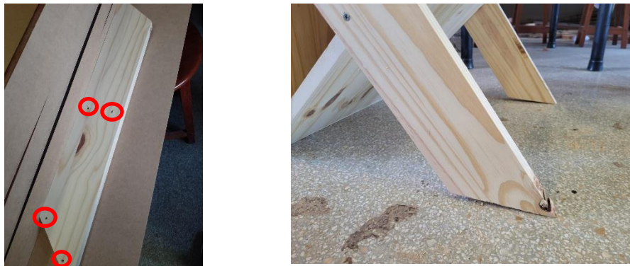
Figure 13: Wood piece with misaligned holes and unstable furniture.
