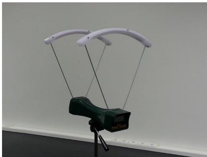
Figure 3. Ballistic chronograph used to measure velocity of diabolo pellets
