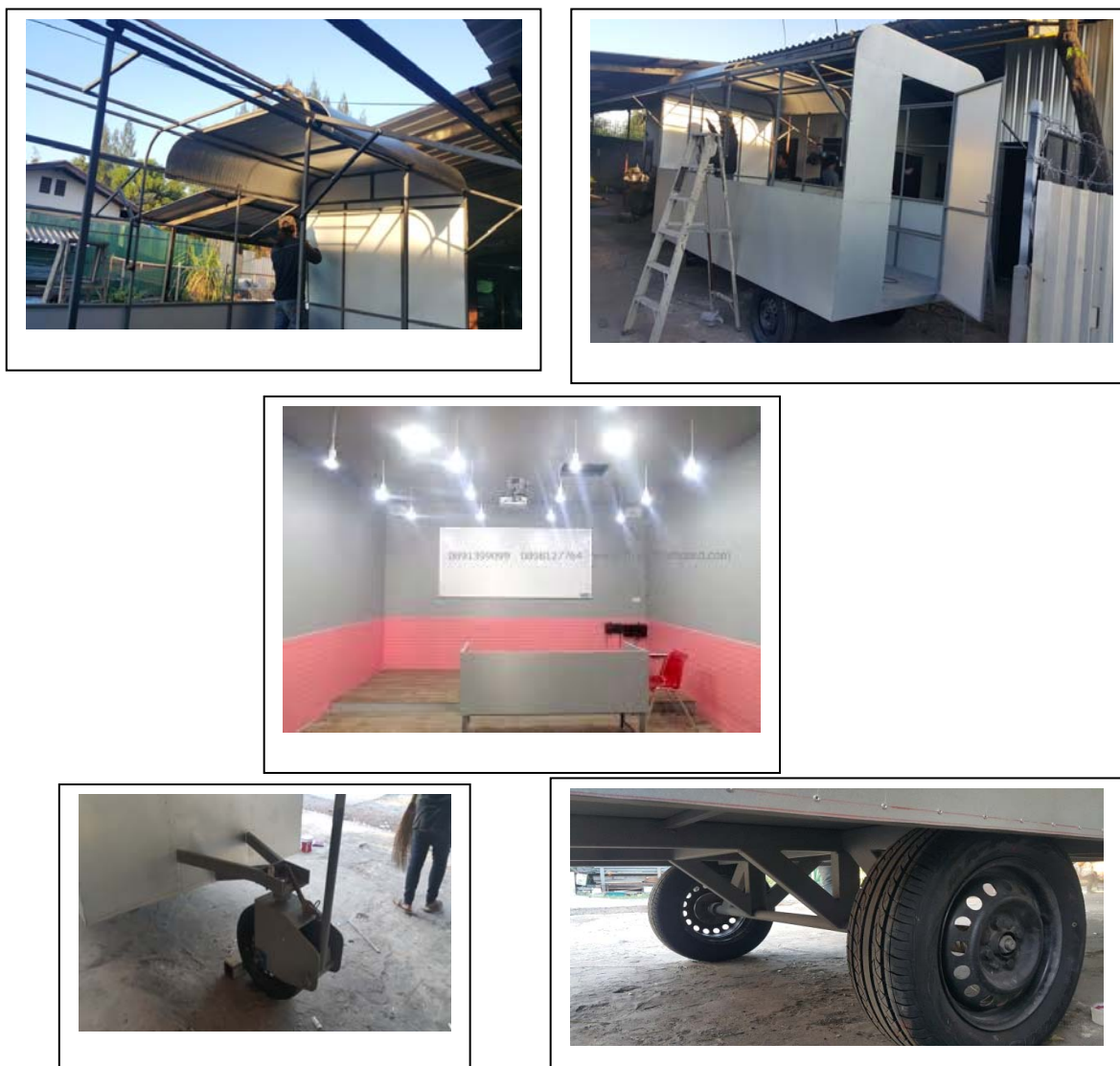
Figure 1 the construction of body, frame and wheels as well as the online mobile classroom
