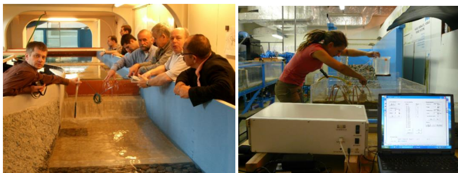
Fig. 2: Measurement on a physical model of a fish ladder on a length scale of 1:20 and pollution transport in soil.
