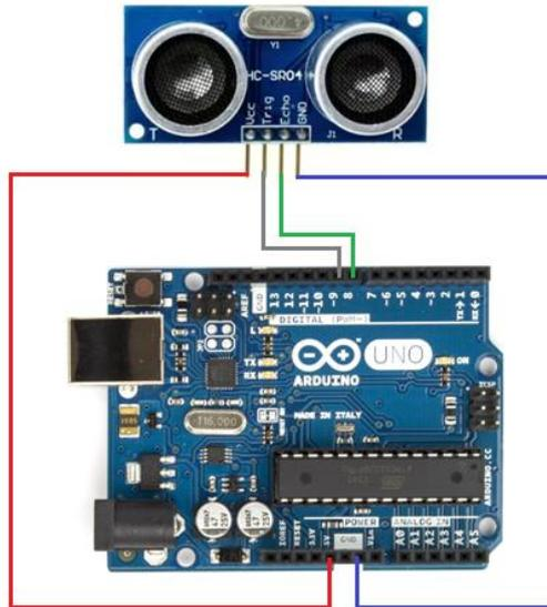
Figure 11: Connection diagram of HC-SR04 with Arduino.
