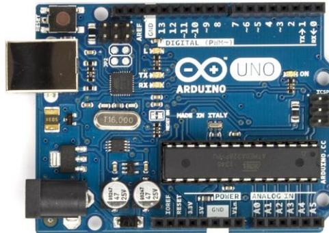
**Figure 1:** The Arduino UNO board.
