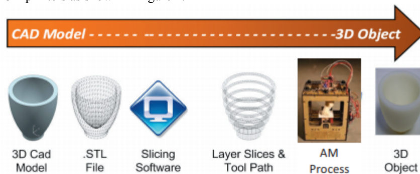
Figure 1. Additive Manufacturing (3D printing) Process (Campbell, Williams, Ivanova, and Garrett, 2011)
